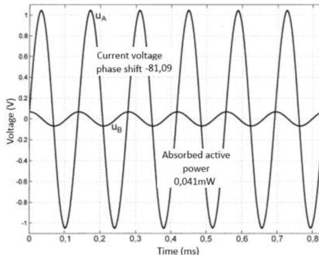
**Fig.6.** Relationship between the voltages  $u_A$  and  $u_B$  for an over-seasonal supply voltage frequency (7212 Hz).  $P = 41 \mu W$
